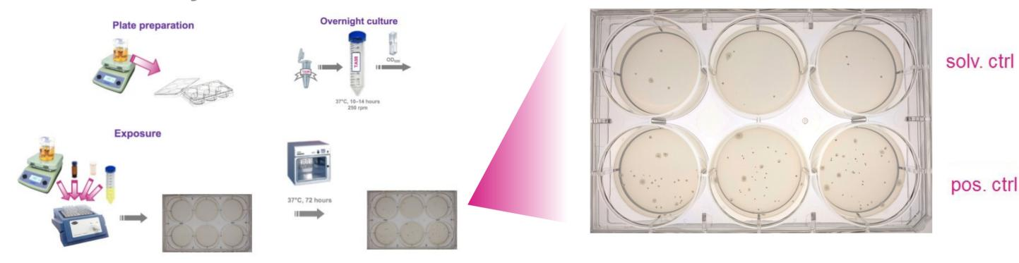
The Xenometrix Ames MPF<sup>™</sup> 98/100 is a microplate fluctuation assay to test mutagenic potential of chemical compounds.
